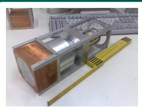
Reduced voltage readout to counteract PMT saturation
